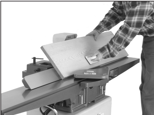
Figure 26. Typical bevel cutting operation.
